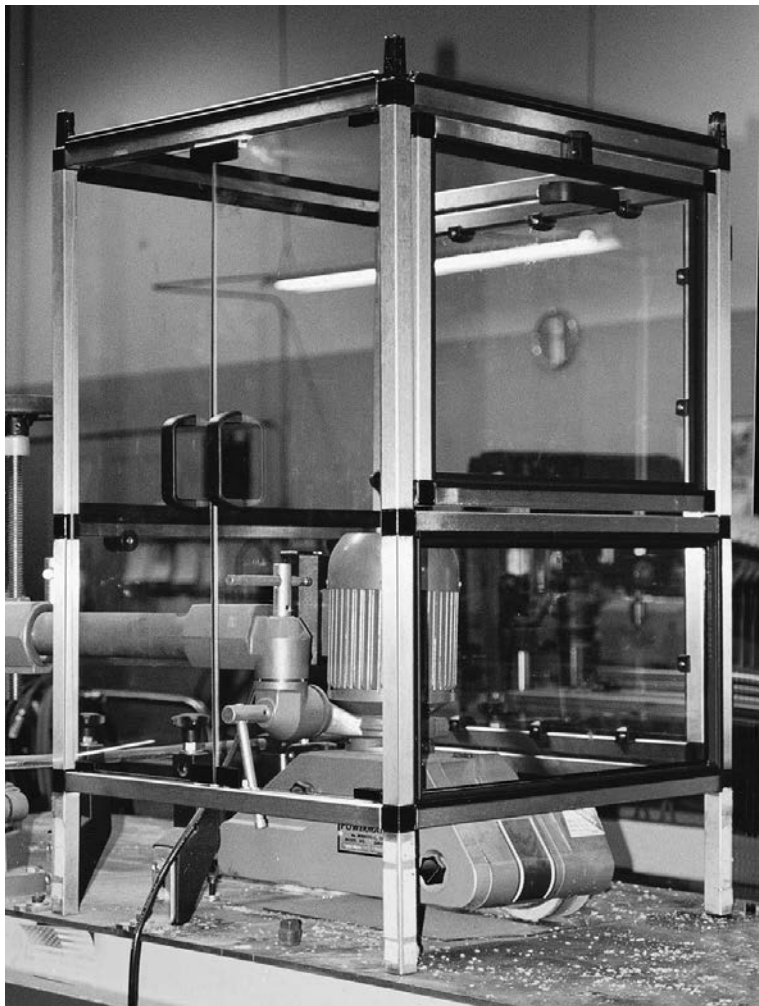
Unframed panel doors on this SpeedFrame enclosure provide economical machinery access.
