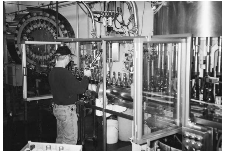
Bifold doors on this free standing enclosure provide easy and unobstructed access to this bottling line.
